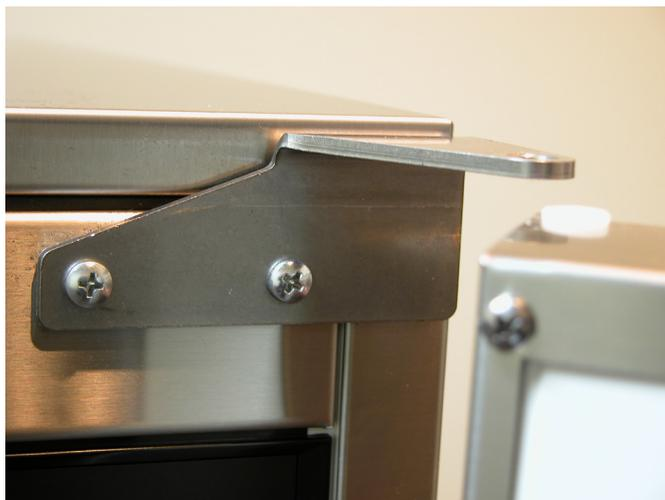
3. Remove two screws and top hinge.
