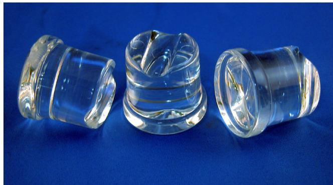
Normal cubes are tapered cylinders. If the cubes are ragged and mis-shaped, mineral scale must be removed from the ice making system
